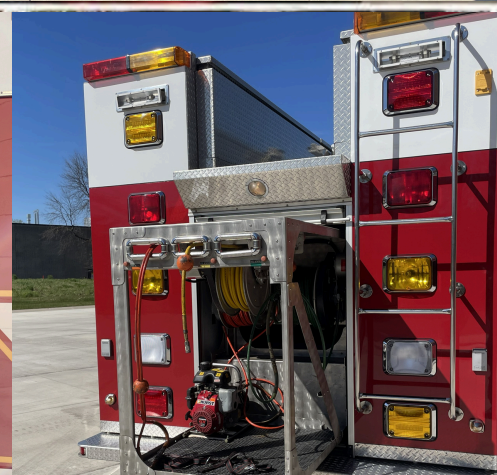
REAR PULL-OUT COMPARTMENT FOR EXTRICATION TOOLS HYDRAULIC & AIR REELS
