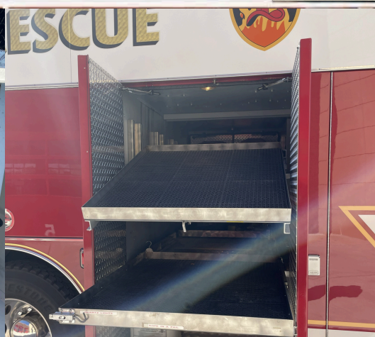
ROLL OUT/TILT DOWN SHELVING 2 TRANSVERSE COMPARTMENTS
