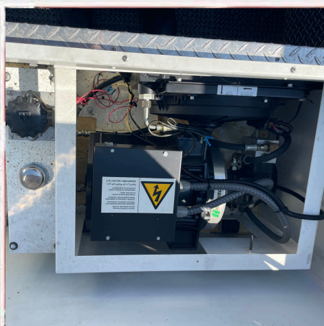
15,000-WATT PTO DRIVEN HYDRAULIC GENERATOR (2) 150' Cord Reels
